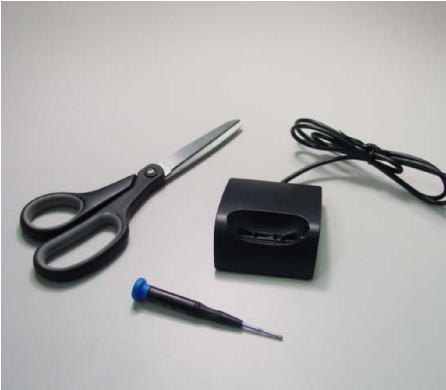
Centro product and tools needed for disassembly – Scissors and Small Phillips Head Screw Driver
